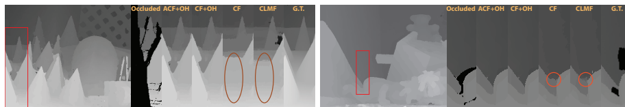
Fig. 5: Depth estimation using cost filtering with and without our OH method on the Cones (left) and Teddy (right) Middlebury benchmark datasets. For each dataset, the left-most figure shows the depth map computed by our method (ACF+OH). The other columns show a close-up of the section highlighted as the red rectangle. Ocluded column shows the depth map computed by ACF without any post-processing. ACF+OH post-processes depth computed by ACF using OH. Similarly, CF+OH indicates the result of CF after post-processing using OH. CF and CLMF show depth maps computed by these algorithms, respectively. The last column shows the Ground Truth (G.T.). Ellipses in CF and CLMF indicate regions that exhibit large errors.
